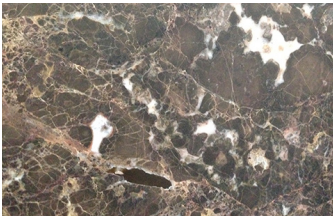
EXAMPLE OF GRAIN AND SHAPE OF THE SLAB WITH FILLING
